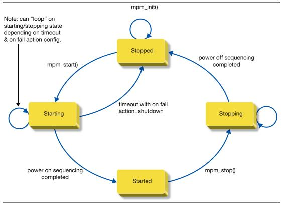
Figure 4-1 • MPM State Transition Diagram
