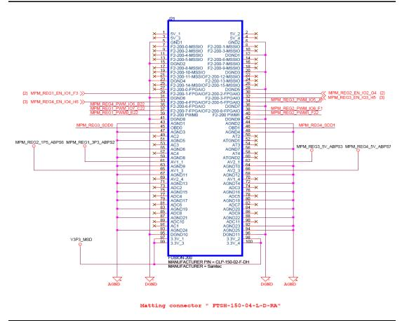
Figure 6-7 • Mixed Signal Connector on MPM DB for Interface to SmartFusion Board
