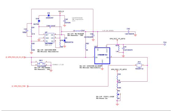
Figure 6-4 • MPM Switching Power Supply 1.5 V
