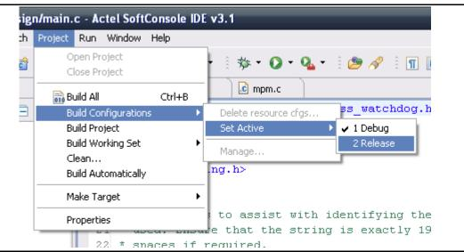
Figure 2-1 • Setting Active Build to Release in SoftConsole
