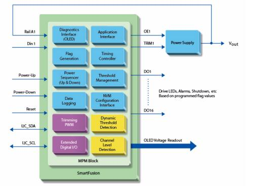
Figure I-1 • Typical System-Level Diagram
