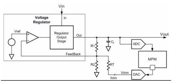
Figure 5-2 • Closed-Loop Trimming Using SmartFusion MPM
