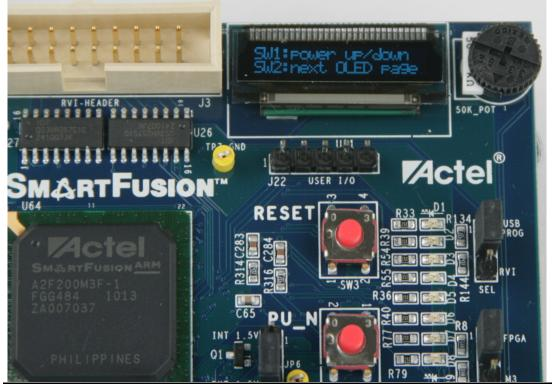
Figure 1-1 • OLED Message After Successful Programming
