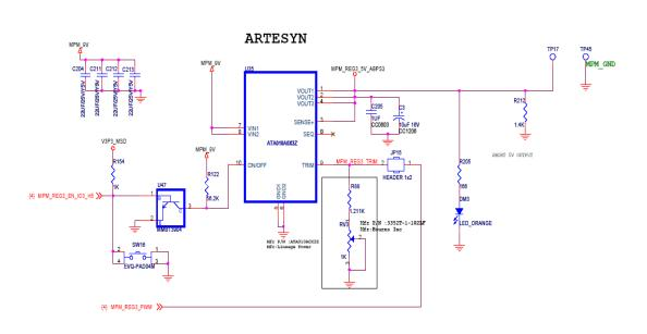
Figure 6-5 • MPM DC-DC Power Supply 5 V
