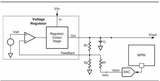
Figure 5-1 • Open-Loop Trimming Using SmartFusion MPM
