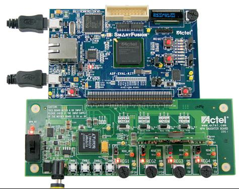
Figure 1-2 • MPM-DC-KIT MPM Daughter Card Attached to SmartFusion Evaluation Kit
