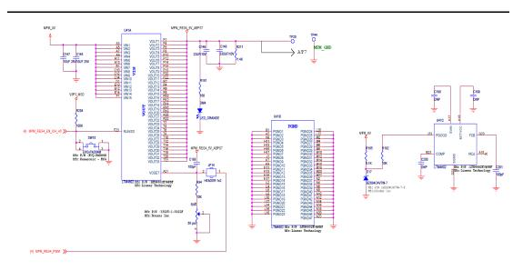
Figure 6-6 • MPM DC-DC PowerSupply 5 V
