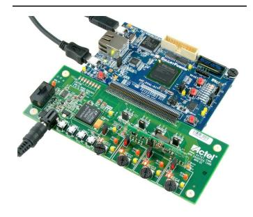
Figure 2 • Mixed Signal Power Manager Daughter Card Kit (MPM-DC-KIT) connected to SmartFusion Evaluation Kit (A2F-EVAL-KIT)
