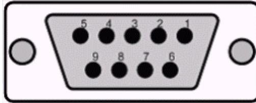
Figure 3 – Serial connector (looking at back of modem)
