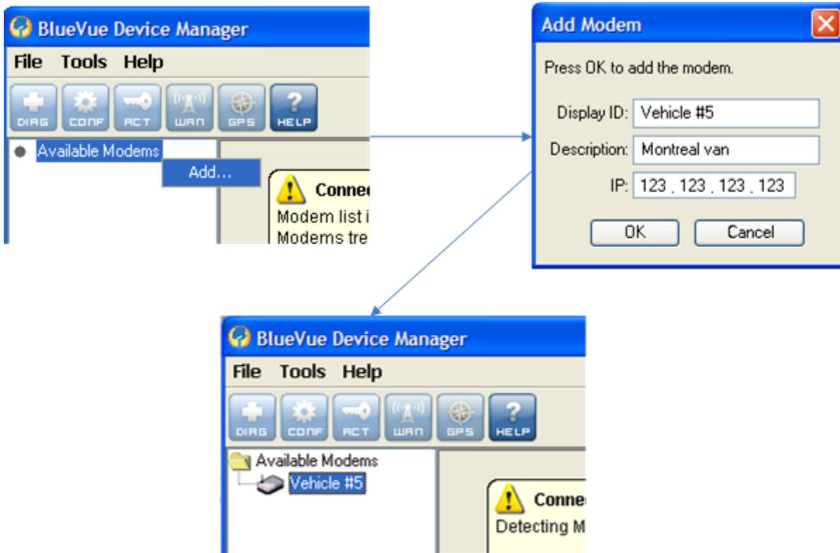
Figure 5 – Connecting to a remote modem
