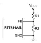
Figure 1. Setting the Output Voltage
