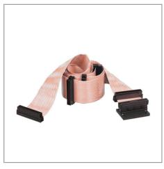
**Description**Introducing Tripp Lite's internal SCSI Ultra2/U160 4-drive LVD ribbon cable with an active U160 terminator. This cable measures 45 inches in length and is made with twist and flat cabling. Because the cable is backwards compatible, it will support SCSI 1,2 & 3 devices such as CD-ROMs and Hard Drives. All Tripp Lite SCSI products regardless of the SCSI generation meet the latest SCSI specifications of ANSI (American National Standards Institute).
