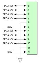
**Figure 12 - Pmod Connections**
