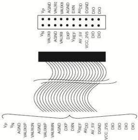
Figure 13 - Analog Header Pin out
