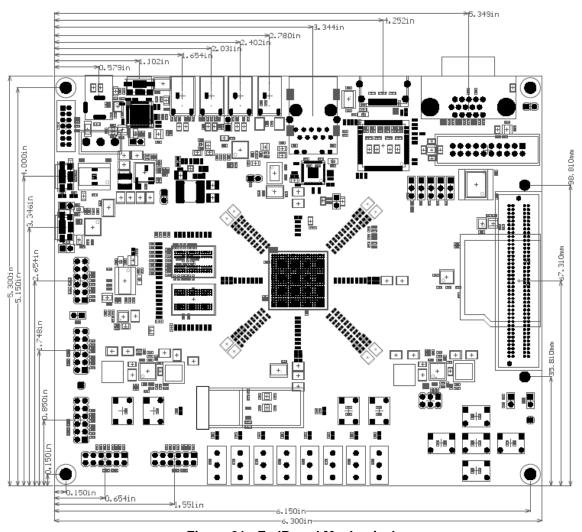
Figure 21 - ZedBoard Mechanical
