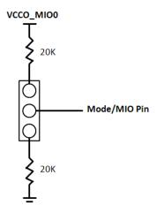
Figure 15 - Configuration Mode Jumpers
