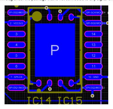
Figure 5 - Overlying Packages for SPI Flash
