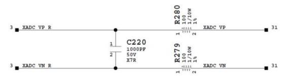
Figure 14 - Anti-Aliasing Filters for XADC Inputs
